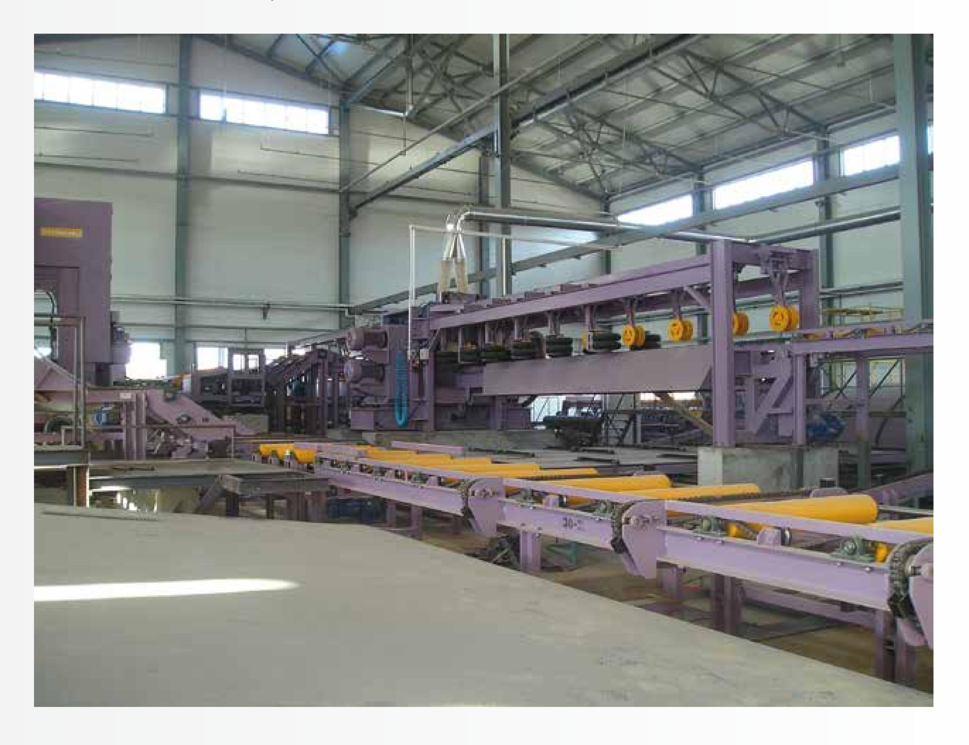
ÜSTÜNKARLI develops semi-automatic sawmills with only two operators. A semi-automated sawmill is not equipped for automation only, it is built to have the most efficient layout and allow the largest possible flow of logs and sawn timber. In order to be well adapted and functioned properly, the conveyors are incorporated into installation, so that allows self-disposal of the waste. There are many plans for automatic sawmills that can be adapted to the special conditions at each installation.
